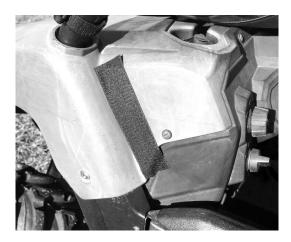
5. Finally, the bottom of the door has three snaps, one on the inside and two on the outside. Best way to put the screw studs in the correct place is to install the screw stud into the snap on the door first. Then pull the door in place and push the point of the screw into the plastic making sure to leave a good mark. Then pull the snap stud out of the door and screw into the plastic where the mark was left. See photo below.
