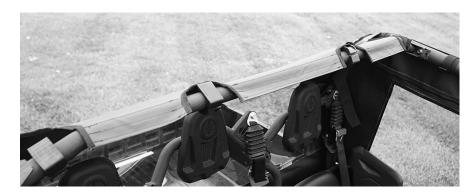
7. The sides of the Rear Window will attach to the Velcro tabs from the doors. The one exception is the top corners that have a double-sided tab that is held in place by a 3" adhesive strip. The bottom of the Rear Window will hang between the bed and the backs of the seats. See the following photos.
