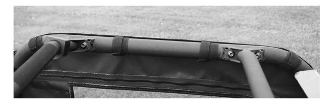
2. The rear edge of the doors has 2 strips of Velcro sewn down the entire length. Starting at the top use the 5" and 21" adhesive strips to attach the door to the roll cage. This attaches to the Velcro sewn down the sides of the rear window. See photos below.
