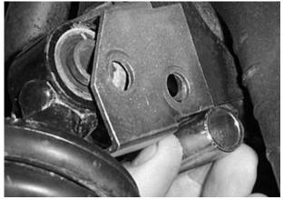
5. Secure the bracket to the ATV using the 10 x 55 hex bolts and 10mm nuts.
