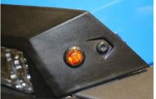
5. Run the short front harness from the front LED lights to the control box and plug into mating connector. The Green wire harness goes to the right/passenger side and the yellow wire harness goes to the left/drivers side. Both green and yellow wires are positive and go to the black wire on each side, the white wire goes to white. Secure the harness with the provided cable ties. NOTE: Black wire is positive and the White is ground, they will not work if reversed.
