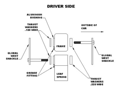
Note: Shackle halves are installed as follows: The bolt on the outboard shackle half goes through the frame and the bolt on the inboard shackle half goes through the spring eyelet bushing.
