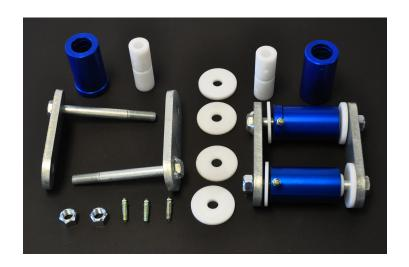
We recommend that a competent shop install this bushing and shackle kit. Presswork and special tools are required to install this kit.
