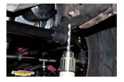
9. For drilling the holes on the side of the frame you will require unbolting the bumper brace.
