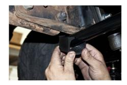
6. Install the bracket next- slide the bracket over the bushing.
