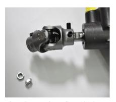
stops. Now turn the input shaft the other direction, counting the number of revolutions
