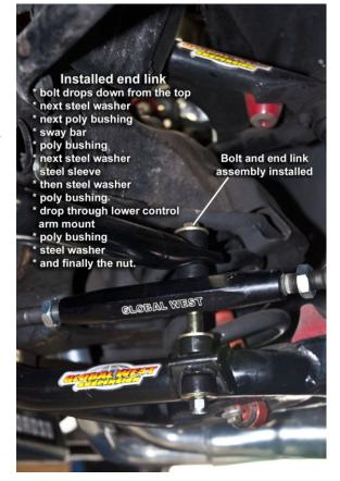
of the steel sleeves onto the bolt, next one steel washer, one poly bushing, and slide the
