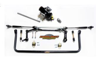
box) one direction until the gear hits the internal stops. Now turn the input shaft the other direction, counting the number of revolutions until it stops again, rotate the input back ½ the number of rotation and the box will be centered.
