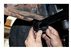
6. Install the bracket next- slide the bracket over the bushing.
