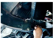
10. Once you have the bottom holes drilled you are going to mark the side of the frame and drill a hole for access. Mark the side of the frame directly above the bottom hole you just drilled. Measure up from the bottom of the frame 1-1/8 inches.
