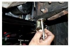
With the sway bar positioned properly mark the frame on both sides of the bracket.
