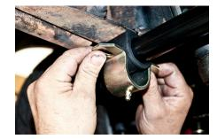
7. You are going to mark the slots on the frame for drilling purposes.
