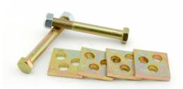
Lockout kits eliminate the lower control arm eccentric. The eccentric adjusts the alignment of your vehicle. It is the bolt that holds the lower control arm to your frame. By turning the eccentric, camber is adjusted (the tilt in or out of the fender) but will also affect caster and toe. Eccentrics because they are an offset cam, have a tendency to slip during suspension movement. When they slip your alignment is lost.
