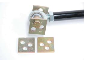
When installing the plates in the rear end bracket from the rear looking forward --- use the bottom hole about in the middle of the plate. # 3 You will be able to read it. Place the  $\frac{1}{2}$  inch bolt supplied in your kit through the plate. Take the strut rod (the side with the steel sleeves with  $\frac{1}{2}$ inch hole in them) up into the bracket. Slide the bolt through the enter assembly.
