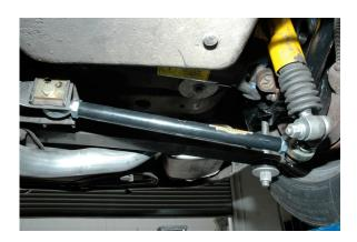
10. Follow the same procedure for the other side. Once both sides are complete you will require a rear wheel alignment. The alignment is handled by loosening the jam nuts on the strut rod and turning the strut rod. Once the alignment is achieved tighten down the jam nuts locking the strut rod in place.
