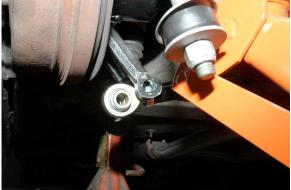
8. Slide the factory shock pin through the assembly and install the slotted hex nut. Tighten the nut down to 80 foot pounds.
