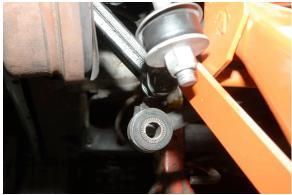
5. Installing the new strut rod kit is relatively easy. You will notice in the photo to the right that the plates are number 1 through 6. The numbers allow you to move the bolt in or out depending on what alignment and the amount of threads showing on the rod ends. For the most part use hole number 3 on both plates.
