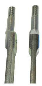
Note: The shaft on the right is a straight shaft (standard) The shaft on the left is offset #702. The offset shows a shift to the left. That should be towards the wheel.
