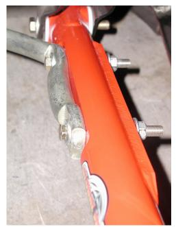
Torque the sway bar to frame bolts to 45 foot pounds.
