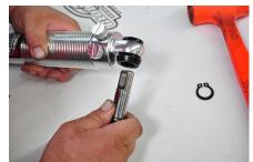
15. Next install the steel sleeve in the bushing, place grease inside the bushing and around the pin. We recommend synthetic grease like NEO Z-12, however any water resistant synthetic grease will work.
