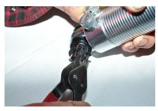
13. First remove the bar from the base of the shock. Almost all the shock companies make something similar. They have a c-clip on each side of the bushing.
