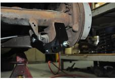
D. Use a drill with a  $\frac{1}{2}$  inch drill bit and drill a new hole through the differential lower arm mount.
