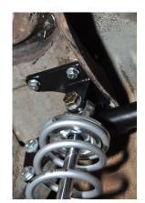
9. Install a  $\frac{1}{2}$  x 20 x 3  $\frac{1}{2}$  bolt with a 12mm flat washer through the lower shock mount. The adjusting knobs need to be on the positioned towards the inside of the car.
