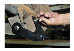
8. Install the shocks starting with the upper mount. Use a  $\frac{1}{2}$  inch x 20 x 3  $\frac{1}{2}$  inch long bolt with a 12mm flat washer and slide it through the upper shock mount. Hold the
