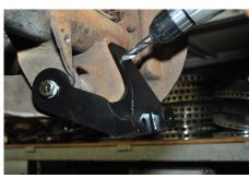
E. Install another  $\frac{1}{2}$  x 20 x 1  $\frac{1}{4}$  bolt with a 12mm flat washer on each side and torque to 70 foot pounds.
