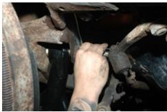
and hardware. Position the eccentric by rotating the bolt until the bolt appears to be about in the middle of the slot. Torque the 9/16 bolt to 120 foot-pounds.
