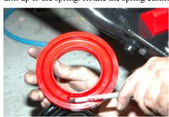
will index with the spring. Use a floor jack under the lower control arm to help hold the arm close to the spring. The floor jack should be positioned towards the ball joint side, not directly under the spring pocket.
