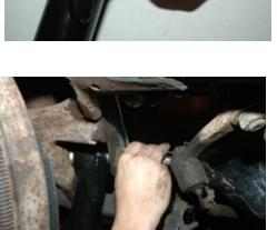
in the frame. The dowel will drop out and should be used on the other side for installation. Keep the dowel in your toolbox. You may need it someday. With the eccentric bolt through the frame, finish stalling the eccentric cam washer and hardware. Position the eccentric by rotating the bolt until the bolt appears to be about in the middle of the slot. Torque the 9/16 bolt to 120 foot-pounds.
