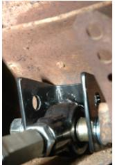
you are using a stock upper control arm. If you are using Global West's Part # TBC-50, install the arm in the lower hole. Use a 5/8 flat washer, locknut and torque to 90 foot-pounds on the frame side only. Do not torque the rear end side till the rear suspension is fully loaded. If you are using a stock upper control arm you cannot torque either side till the full weight of the car is resting on the rear end.
