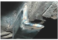
6. After the tacking process is complete, weld the subframes to the rails.
