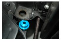
7. Install the female portion of the bushings located at the firewall and radiator core support. The bushing indexes on the step of the installed male bushing and sandwiches the frame. Basically when the assembly is tightened, the bushing halves will lock the frame in position so it cannot slip.
