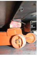
between the frame and body allow you to remove the old bushings and install the new.
