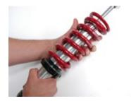
D. On top of the spring you will install a small stepped ring. The ring will index inside the spring.
