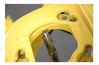
8. If you have ordered a negative roll system you will have an upper control arm template for drilling different locating holes. Note: If you did not order a negative roll system no template will be provided but you will have to drill the upper mounting holes out to 9/16 diameter. The original holes are ½ inch diameter. Slide
