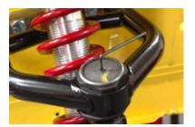
18. Hook up your steering and the sway bar. Many times it's easier to put the sway bar end links on after the cars ride height is set and on the ground.
