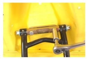
you do not have a negative roll system you will not have the plate. Just bolt the upper control arm direct. Tighten the control arm bolts to 90 foot pounds.
