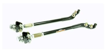
strut rod to the lower arm). These bolts replace your factory bolts that attach the strut rod to the lower control arm. You will have to open up the bolt holes in the lower control arm to 9/16 for installation. If you are unsure how to remove the factory strut rods, a service manual will help if a procedure is required.
