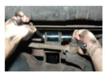
during assembly. Swing the arm into position and using new hardware, install the bolt with a flat washer against the head of the bolt and one
