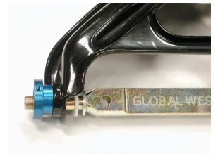
4. Press the aluminum bushings into the control arm, making sure that the hole for the grease zerk fitting is positioned in such a way that you will be able to access the zerk for lubrication purposes once the control arms are installed on the
