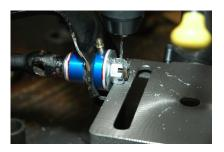
12. Install a cotter pin after drilling.
