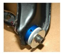
10. Install the slotted hex nut and tighten down the nut until there is thrust contact between the inner and outer thrust surfaces. You will run the nut to set the bushing and thrust washers. After they are seated, back off the nut and slightly tighten the
