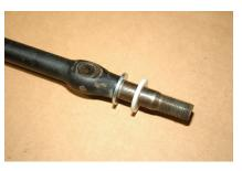
way on. Next install one of the inner plastic thrust washers. Install the thrust washers on both side of the shaft.
