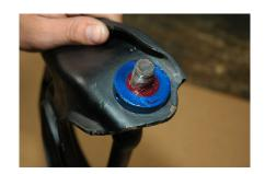
8. Lubricate the inside of the plastic insert and install into the bushing. Sometimes you may have to slightly tap the insert down into the housing in order to get the outer thrust washers and nut on.
