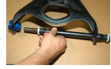
7. After the bushings are installed, lubricate the housings in the arm with good water resistance grease. Synthetic works well. We recommend neo z-12 but any synthetic grease will work.
