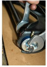
nut down till you have thrust contact, then go 1/8 of a turn more or one flat on the nut. (You are adjusting the bushing as though it was a wheel bearing).
