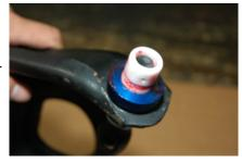
9. Install the plastic outer thrust washer and then the steel outer thrust washer.
