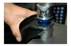
4. Next you are going to install the cross shaft into the arm. Before you do install one of the small steel inner thrust washers on the shaft and slide it all the
