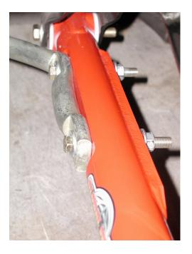
Torque the sway bar to frame bolts to 45 foot pounds.
