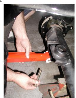
sway bar can be positioned correctly. First slide the sway bar up into position
