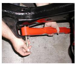
end attaches to the frame, each bearing will have two steel spacers located one on each side of the spherical bearing. They are already installed. Note: The recess in the control arm goes to the inside of the car. Simply slip the arm with the spacers installed up into the frame. Make sure the grease fitting on the rear end side of the arm is facing down towards the ground. Slide the stock bolt through and torque to 70 ft/lbs.
