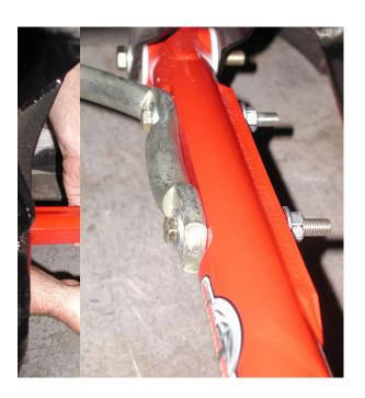
Torque the sway bar to frame bolts to 45 foot pounds.
