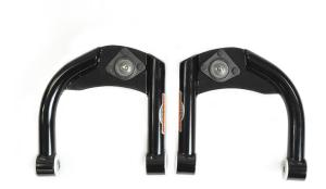
CTA-32 and CTA-32D are pre-assembled. Both upper control arms will bolt directly into the stock upper arm bracket. Make sure that the grease fittings on the control arm are facing down when bolted into the upper bracket. The bushings are pre-lubricated; you will have to lubricate the upper ball joint after installation on the spindle.
