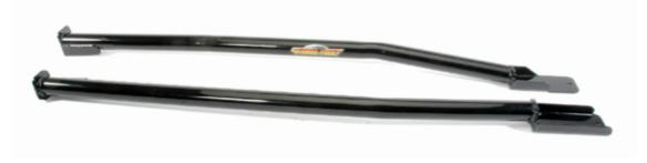
905 Subframe connectors will connect into the floor bulkhead supports. There is a right and a left subframe. The subframe when installed will follow the contour of the floor and tuck up inside the outer rocker rail. They will not hang down or be seen once they are installed. Based on the photo – the top subframe is the driver side.
