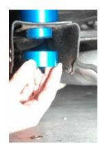
9. Install a 5/8 x 3-1/2 bolt with a 5/8-lock washer and 5/8 flat washer and install at the firewall location. Do not tighten yet.
