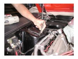
Take the template and align the holes so they locate in the narrow slot where the carriage bolts index. Center punch the inside hole first. Do not center punch all the holes at this time.
