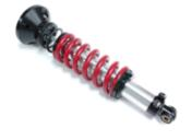
adjusting the collar up to about 3 ¼ inches from the top of the shock where the threads start down. This can be done after the top and bottom of the coilover is mounted to the car.
