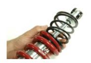
F. The upper shock spring cap slides over the shaft as shown to the right.
