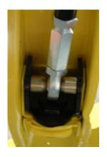
10. Install the new tubular lower control arm. The control arm has a gold steel spacer on each side of the bearing. Make sure they are there and not setting in the box. The spacers make up the
