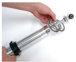
B. Next install the needle bearing kit onto the shock collar. First slide one thin washer over then the bearing and then the last thin washer. Do not lubricate the bearing. The lube will collect dirt over time and stop the bearing from rotating.
