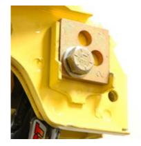
plate 3 ways or flipping the plate over and rotating 3 ways. To start, we use position marked 1 facing the front of the car. Slide the bolt through the plate, through the lower control arm and into the other side of the frame rail.
