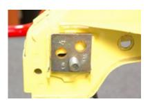
11. Time to bolt the lower shock mount, strut rod, and the lower arm together. The shock mount has 3 bolts welded to it. You will slip the lower shock mount through the strut rod and then place that assemble into the lower arm.
