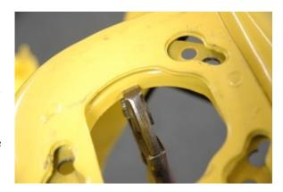
8. Drill the upper control arm mounting holes out to 9/16 diameter. The original holes are ½ inch diameter.
