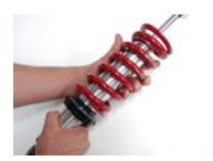
D. On top of the spring you will install a small stepped ring. The ring will index inside the spring.
