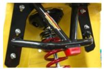
lubricate the ball joint you need to remove the grease fitting and install a plug. This is so the bump stop hits the top of the ball joint flat.
