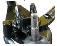
The bolts are 9/16 and ½. Install a ½ inch flat washer and stovelock nut on the ½ inch bolt. Install one 9/16 washer on each 9/16 bolt and
