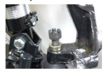
Install as shown and also install the upper ball joint through the spindle.
