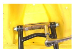
9. Installing the strut rod requires removing the 1-inch nut, lock washer, and flat washer off the pre-assembled strut rod.
