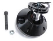
H. Adjust the collar at the bottom of the shock, up until it touches the upper cone for installation. We suggest
