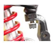
16. After the ball joints are tightened down lubricate the upper ball joint. After you
