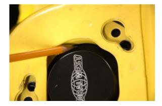
7. Sometimes in order to get the upper mount to fit flat in the tower you may have to bend the lip where the factory spring indexed. The lip bends easily with a vise grip. Once you have the upper mount able to install in the tower we will move onto the upper arm install. Do not install the upper mount yet. (Notice the new holes drilled in the tower from the template.)
