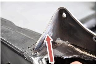
Note: Take your time durning this process. The cleaner the frame rail the stronger and cleaner the welds will be.
