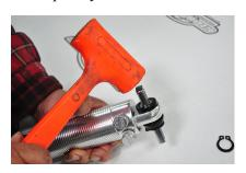
15. Next install the steel sleeve in the bushing, place grease inside the bushing and around the pin. We recommend synthetic grease like NEO Z-12, however any water resistant synthetic grease will work.
