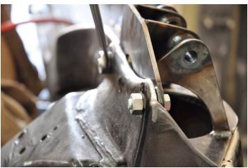
Note: In the picture to the right notice the location of the gusset plate. DO NOT WELD IN THIS LOCATION UNTIL THE GUSSET PLATE IS IN PLACE.
