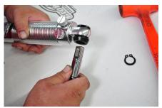
16. The steel sleeve will push into the bushing fairly easy. Push the sleeve in till it bottoms out with the bushing.
