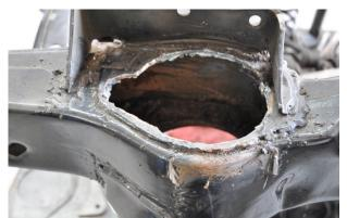
Note: Use a pneumatic cut off wheel or 4" grinder to remove the bump stop. Cut along the welds and try not to cut into the frame rail!
