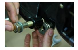
15. Install the aluminum clamps onto the differential. The clamp with the center hole goes on the bottom side of the axle tube. – Do not tighten the clamps down yet. You will have to slide the clamp into position first.
