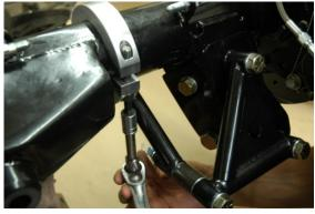
18. Next tighten down the clamps and tighten down the ½ inch bolt holding the short tube. Tighten down the allen bolts so the gap on each side of the rear end is equal. Tighten to 35 pounds. Place a little red loctite on the threads. Torque the ½ inch bolt to 70 foot
