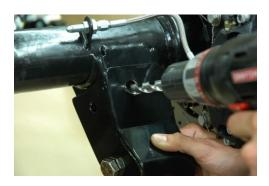
13. Using a ½ inch drill and ½ inch drill bit, drill the side mounting bolt hole. Make sure the bracket is tight up against the rear end mount. You may want to clamp it.
