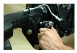
14. Next slide the bottom of the tubular bracket over to the index hole in the new bracket. You may or may not need spacers. If so they are supplied in your kit. You want the bracket to be flat. Using a ½ inch x 20 bolt and flat washer, slide the bolt through and using a ½ x 20 lock nut tighten down the assembly to 70 foot pounds. You can now tighten the upper bolt as well to 70 foot pounds.
