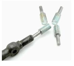
4. Weld the stud to the shaft. We recommend TIG welding. Weld all the way around the shaft filling in the gap. Buff any high welds off so the bushing will slide on.
