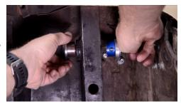
13. Loosen the nut, unthread the plug, and remove the assemble out of the bushing.
