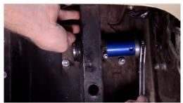
12. Once the bushing has bottomed out, release the tension on the bushing and unthread the plug off of the rod. You will have to thread the rod deeper into the housing so threads protrude at least ½ an inch past the frame. Flip the threaded plug around and thread it back onto the rod. Retighten the nut and finish pulling the bushing into the frame. The bushing will stop when it contacts the threaded plug and will be flush with the frame.
