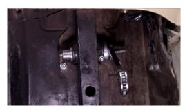
Note: The driver side is similar to installing the frame bushing however the rod will always feed in from the outside of the frame rail. The passenger side is from the inside of the frame rail.
