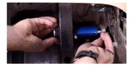
9. Install the steel flat washer onto the threaded rod.
