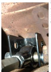
you are using a stock upper control arm. If you are using Global West's Part # TBC-51, install the arm in the lower hole. Use a 5/8 flat washer, locknut and torque to 90 foot-pounds on the frame side only. Do not torque the rear end side till the rear suspension is fully loaded. If you are using a stock upper control arm you cannot torque either side till the full weight of the car is resting on the rear end.
