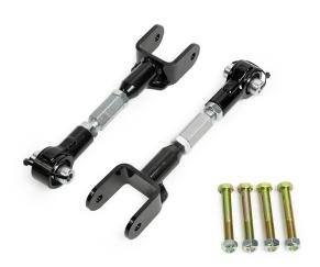
factory arm. Adjust the length of the arm by placing a wrench on the adjusting hex sleeve. This is approximately two inches long located between the jam nuts. Rotating the adjuster will change the length of the arm. **DO NOT** adjust one end of the arm by itself! Use the adjuster. Adjusting one end only will offset the amount of threads required for holding the arm together when installed on the car.
