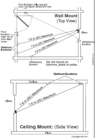
NOTE: If the device is ceiling mounted, the end with the hole (Microphone end) should face the protected glass.
