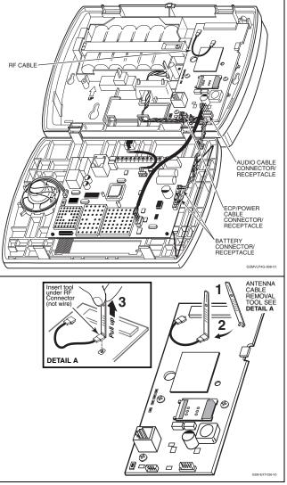
5. Slip the Antenna Cable Removal Tool (p/n 700-03513) under RF Cable connector as shown.
