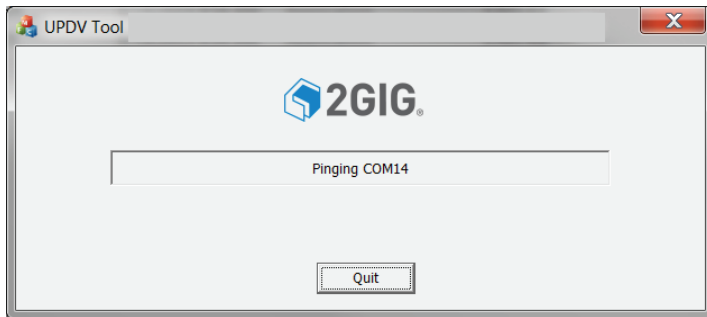
Figure 8. Pinging Active COM Port on PC
