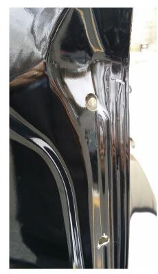
Use the drill locations you just made when you went through the underside of the trunk to locate where you will dremel the opening for the screws. You will need to
