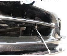
5. Install additional support brackets as needed.
