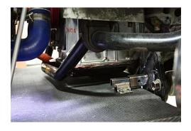
6. Re-install the entire bumper and Splitter assembly onto the vehicle.
