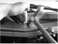
F) Remove Cowl Trim from vehicle. There are 4 plastic pieces to be removed, start with the small parts that are closest to the fenders. Use a short Phillips screwdriver to loosen the center of the fasteners and extract them with a fork tool. Once the 2 small parts are removed the large center parts can be removed, start with the passenger side.
