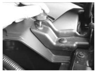
G) Drill two 5/16" holes in Drivers side cowl trim piece. Line up your drill with edge of the rubber seal and approximately 1/2" from the corner of the part. The new squirter hoses provided in the kit will be routed through these holes.
