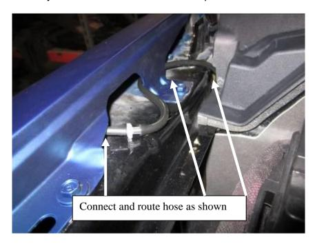
3) Tuck hose and connector inside fender and route neatly up to hinge as shown in pick.
